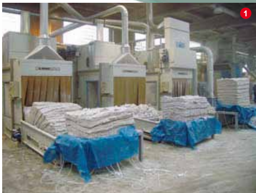
AIRLAY "FELTECH" WITH RESIN DISTRIBUTOR
