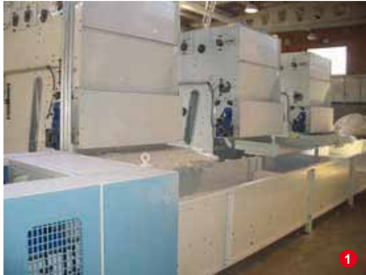
BLENDING LINE WITH CONTINUOUS WEIGHING BALE OPENER "AP TYPE" TO WORK WITH ANY KIND OF FIBRES
