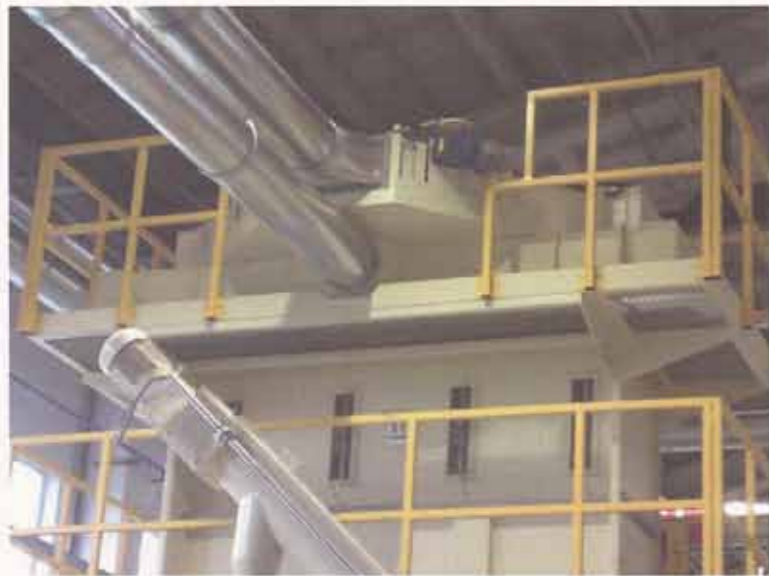
HIGH PRECISION CONDENSER COP-2500 WITH INNER VARIABLE PRESSURE AND AUTOMATIC MATERIAL ROUTER
