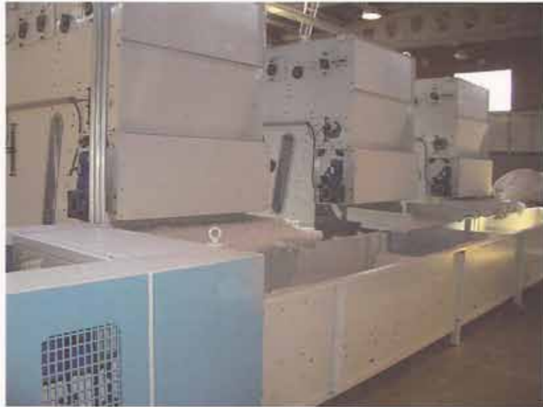
BLENDING LINE WITH CONTINUOUS WEIGHING BALE OPENER "AP TYPE" TO WORK WITH ANY KIND OF FIBRES: NATURAL, RECYCLED AND SYNTHETIC.
