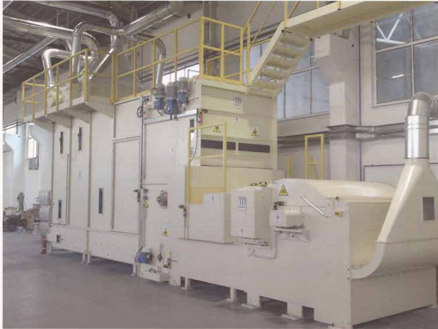
HOPPER FEEDER ABC-1500/2000 UP TO 6 MTS LENGTH, THAT FEEDS THE FIBRES AS A MAT TO THE FINE OPENER MCM-1500-2000/SN
