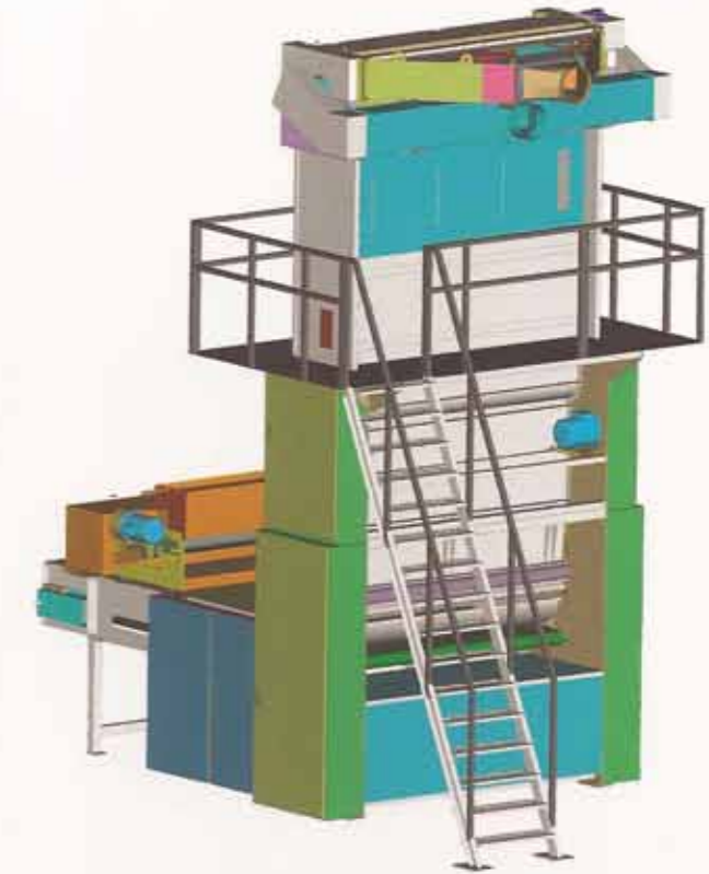
AUTOLEVELER HOPPER FEEDER MODEL CNA WITH CONTINUOUS WEIGHING CONTROL
