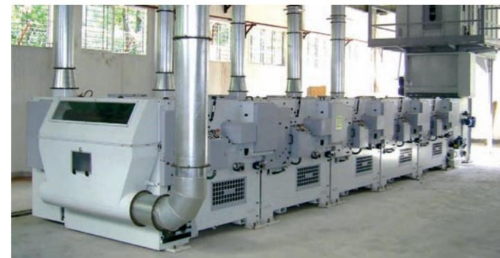
BENJAMIN Recycling Line is available in 1500 mm working width from 1 to 6 drums configuration.
